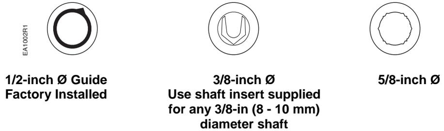
**NOTE:** For all damper shafts with the exception of the 1/2-inch round shaft: Remove 1/2-inch Ø guide before installation.
